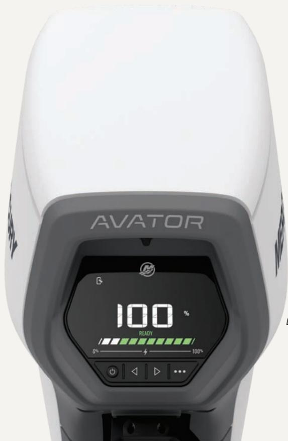
Integrated Outboard Display for Tiller Models
